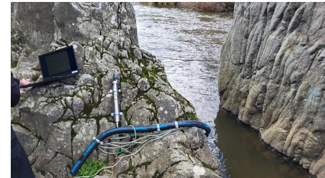
Station hydrométrique continue, @SMTBV
